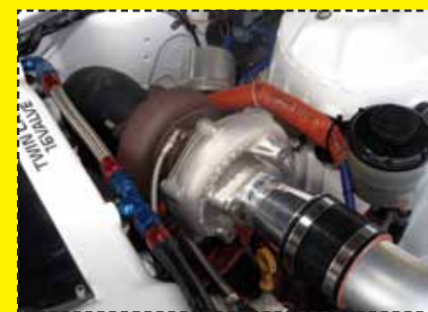
Spot the 36mm restrictor just on the turbo inlet
